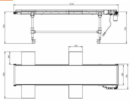
Drawing related to a conveyor belt with a length of 3000 mm and a width of 600 mm; Possibility to customize the belt with different widths (es. 200 - 400 -600 - 800- 1000 mm...etc), and customizable length based on the needs of client.
